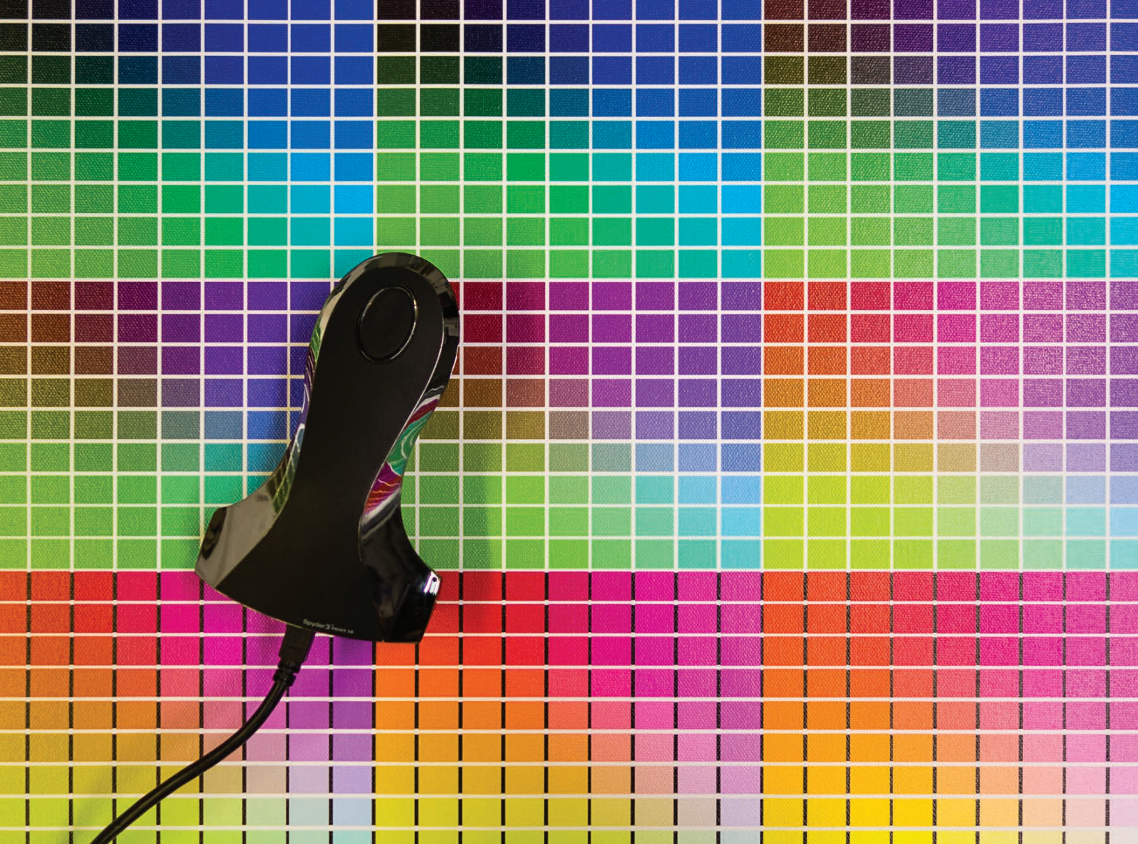
FIGURE 3: A spectrophotometer can be used to scan a target print to create a profile for a specific printer, ink and paper combination.
