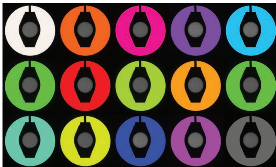
FIGURE 2: As you calibrate your monitor, it will display an array of different colors at different brightness values that are analyzed through the colorimeter and accompanying software.
